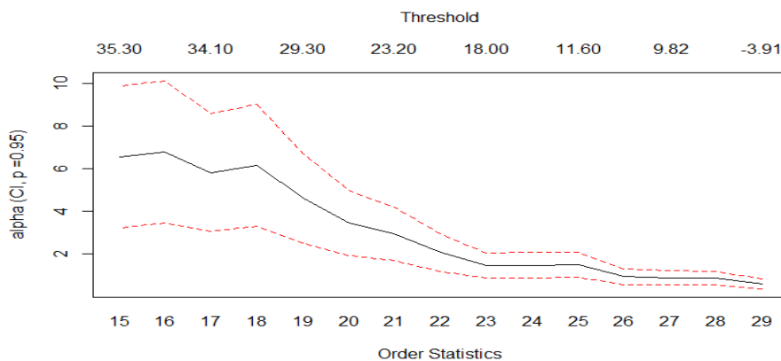
Figure 4.1 : order statistics for Bank of Kigali resulting for fitting the Generalized Pareto Distribution to the monthly data.
